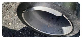
PIPE STIFFENERS CAN EFFECTIVELY PREVENT THE DEFORMATION OF HDPE PIPE AND PREVENT THE OVAL OF PIPE
