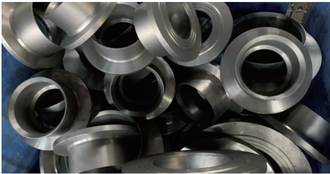
BEFORE SECOND SHOT BLASTING
