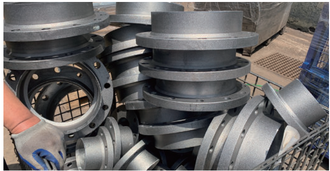
AFTER SECOND SHOT BLASTING
