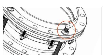
② ONLY 25% QUANTITY(NO LESS THAN 4 PCS) LONG TIE RODS ARE NEEDED, SHORT INSTALLATION TIME AND LOW COST.
