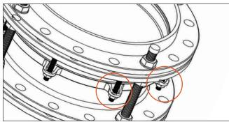
**(1) GOOD SEALING CAN BE ACHIEVED BY** TIGHTENING SEPARATE SMALL BOLTS, NOT AFFECTED BY THE AXIAL FORCE OF THE PIPELINE.
