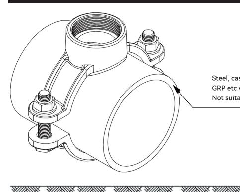
Steel, cast iron, asbestos cement, GRP etc which pipe OD is in our range Not suitable for plastic pipe(PE &PVC pipe)
